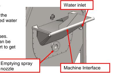
**Emptying spray nozzle** can be connected to a pump, spraying water into the washer drum for an efficient emptying of the drum. Water is normally recirculated from the outlet section to create optimal flow.
