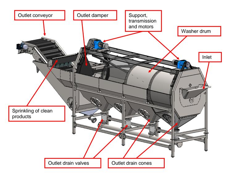
SKALS VTX washing machine is built with modular design. The machine can be delivered with 2, 3 or 4 sections. The washing drum has a diameter of 1400mm. That ensures high capacity and efficient gentle washing of vegetables.
