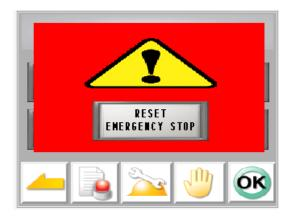
When the emergency circuit is OK the pop-up disappears and the MAIN SCREEN is shown.
