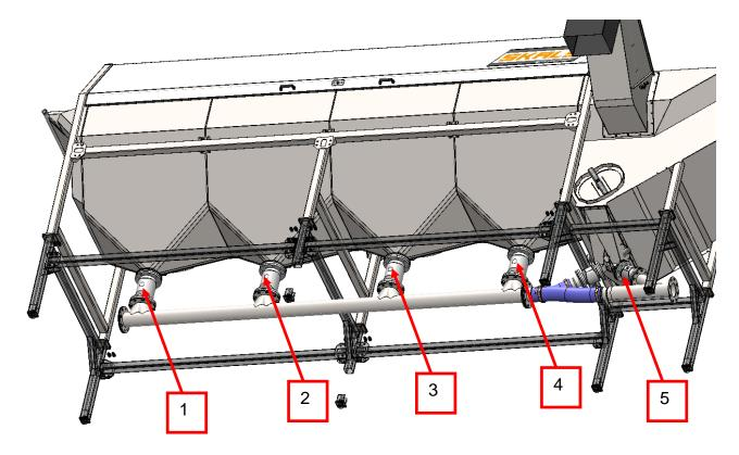
The valves are of the pinch valve type. The valves are activated by air pressure. The valve is "normally open". That means closed under pressure. The valve squeezes the media. If plant residues gets stuck, the valve closes anyway by squeezing arround the foreign.
