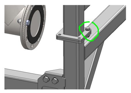
The funnel under the outlet must be mounted with M8 bolts and a gasket.
