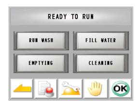
**EMPTYING:** Is used after normal operation to open the outlet damper, and let the machine run for a predefined time until its empty. The time can be set under SETUP
